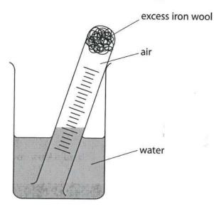
A teacher sets up the apparatus and records the initial volume of gas in the tube.
