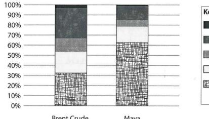
Key Refinery gas Gasoline Kerosene Diesel Fuel oil and bitumen
