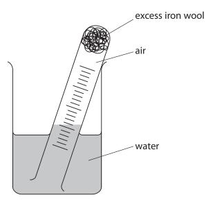
A teacher sets up the apparatus and records the initial volume of gas in the tube.
