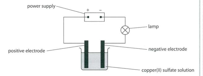
Copper forms at the negative electrode and oxygen forms at the positive electrode.
